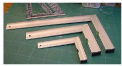
Accurate engineering squares are a must. Cheap (~\$12) but quite accurate set of 3 squares at Harbor Freight. Alternately; plastic carpenter squares. Joe trims the corner flange of the square. The carpenter square enables clamping. Clamps are useful in both
