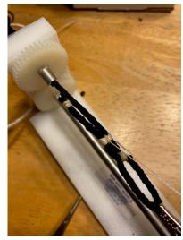
Dan also demonstrated various types of seizing. A throat seizing is used to fasten overlapping rope. If the line is cable laid, loop the ends to the left and under the standing part. If the line is hawser/shroud laid, loop to right and under standing part. Camp into the server. Add a stop knot (double overhand). Tie the loop (Common Whipping). Adjust the loop around the deadeye. Set the seizing with acrylic floor finish.
