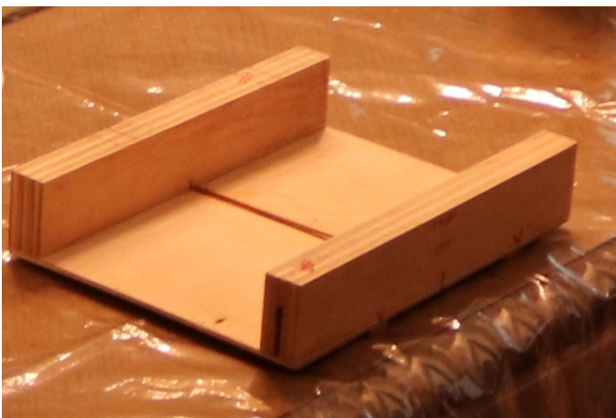
Indexing slide for cutting. Note the strip for maintaining the spacing between cuts
