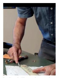
Turn the paper over and on the grid side of the paper. Use a pounce wheel guided by a ruler to indicate rivets .Make sure the wheels aren't to sharp so not to put holes in the paper. Place a magazine underneath the paper. If the table surface is to hard the pounce wheel will put holes in the paper . A magazine underneath will prevent that.
