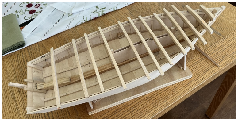
Beginning of deck beams with a camber
