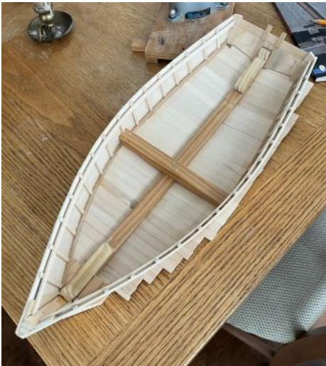
bottom planks, rough chunks at the bow, neither cleaned up or trimmed (top)
