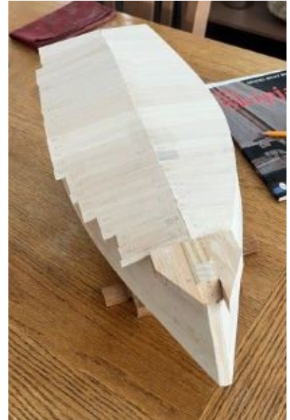
bottom planks, rough chunks at the bow, neither cleaned up or trimmed (bottom)
