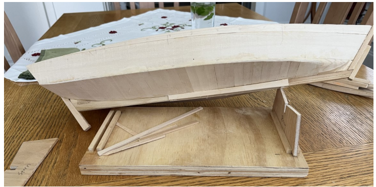
keel and slot for centerboard installed. Bow chunks cleaned up
