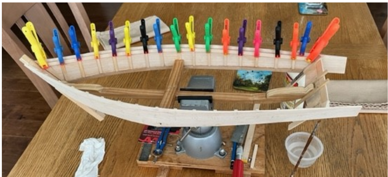
Side planks and frames attached. The strongback, used to spread the width of the boat at midship. This will eventually be removed
